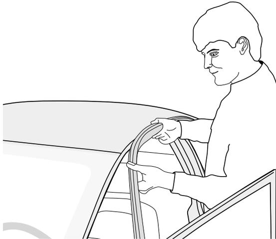
**GB** Unscrew the 10 TORX screws which keep the plastic moulding in place. Bend the moulding out a bit as shown in the picture.
